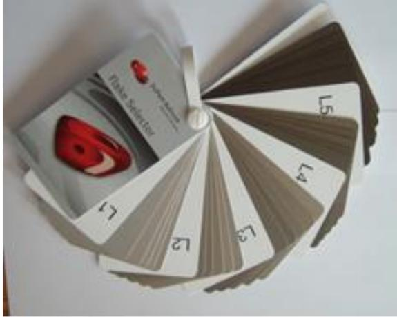
The Flake Selector shows mixtures of aluminium pigments (silvers) in different levels of coarseness. The set is divided in five Lightness Groups (L 1 – 5). Within each Lightness Group there is one chip for each effect level (E1 – E5).
